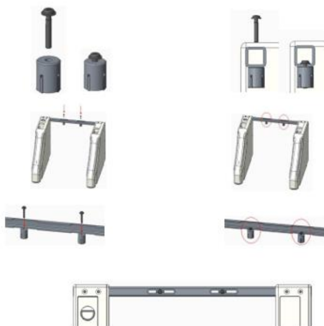
Figure 7: The equipment is attached to the toilet with bolts
