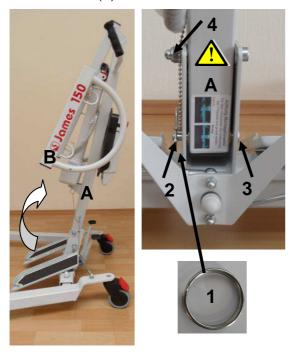
By inserting bolt (3) into the borehole, the column (A) is arrested.
